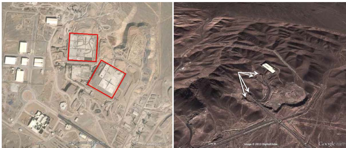
Figure 8. Iran's Natanz enrichment plant (left) under construction in 2003, with the now buried centrifuge halls shown in red outline, and the Fordow enrichment plant (right) in 2012 with arrows indicating four tunnel entrances. In both cases, the centrifuge halls are underground for protection from attack. Both plants are under IAEA safeguards. Source: Google Earth.
