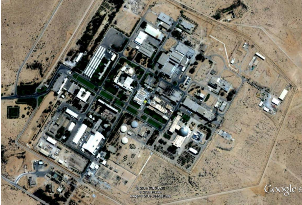
Figure 2. The Negev Nuclear Research Center near Dimona, Israel. The reactor under the dome at the lower right is believed to have produced plutonium for Israel’s nuclear weapons, with the plutonium being separated in an adjoining underground reprocessing plant. The complex may also host a small gas-centrifuge uranium-enrichment plant. Source: Google Earth.
