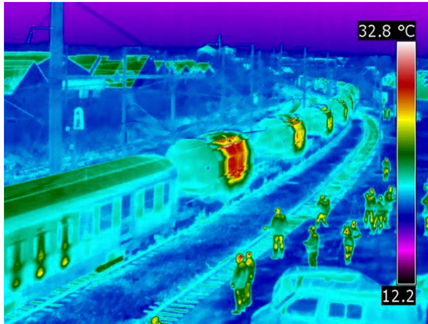
Figure 3. The sensitivity of thermal imaging is demonstrated by the hot spots seen on the outside of rail cars carrying containers of hot glassified nuclear waste being transported from France to Germany. Source: Greenpeace.
